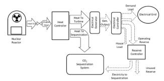
The amount of heat and electricity carried to the iCLEAR<sup>™</sup> process will vary as the flow from the plant is modulated to optimize the value of the plant output and minimize operating cost.
